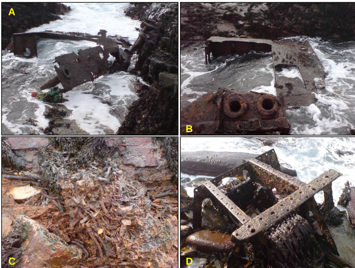
PLATE 21: DISPERSED PONTOON DEBRIS AT HOXA: A AND B) FRAGMENTARY REMAINS OF A PORTION OF PONTOON SECTION; C) CORRODED NET/WIRES; D) WINCH MECHANISM
