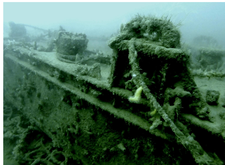
A: Machinery on RC1 showing fairlead, post (with wireguide) and pulley
